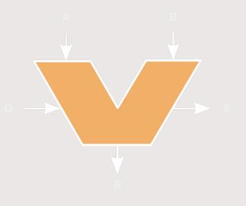
The ALU combines multiple full adders and additional logic circuits to perform arithmetic and logical operations (AND, OR, XOR and even more)
